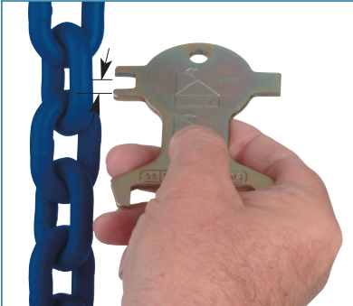
Inspection of material diameter
